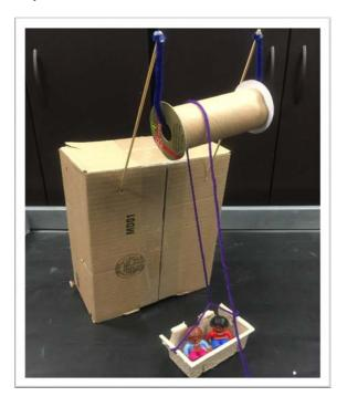
Escalator - moves an object up an inclined plane by having the 'floor' move
