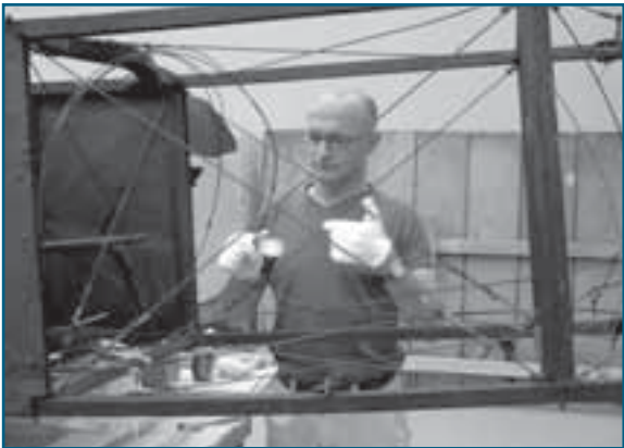
Conservator reassembling wire rigging located on the Borel-Morane Monoplane's fuselage
