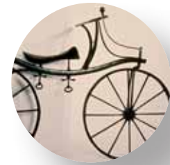
This Johnson Hobby Horse (or draisine) was built in 1818. Propelled by the rider's feet, this ancestor of the bicycle is on display at the Canada Science and Technology Museum. CSTMC—1981.0202
