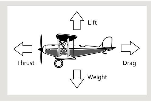
Lift is the force that pushes an airplane upwards, and must be greater than the force of weight for a plane to fly. Lift is generated primarily by a plane's wings.
