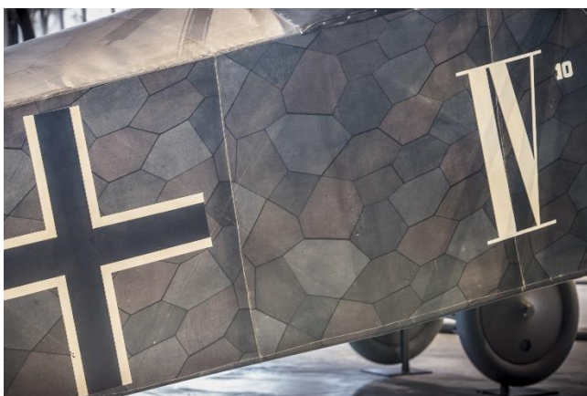
Image 2: Side view of an A.E.G. G.IV bomber. Note the polygon pattern used for camouflage purposes.
