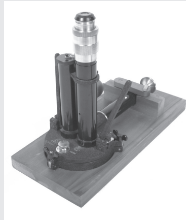
Figure 34: A Bausch & Lomb konimeter from the Gage Institute collection. This instrument was used in occupational health research to measure the quantity of inhalable dust in the environment. (UTSIC collection no. 2016.phlt.1.104.1-6)
