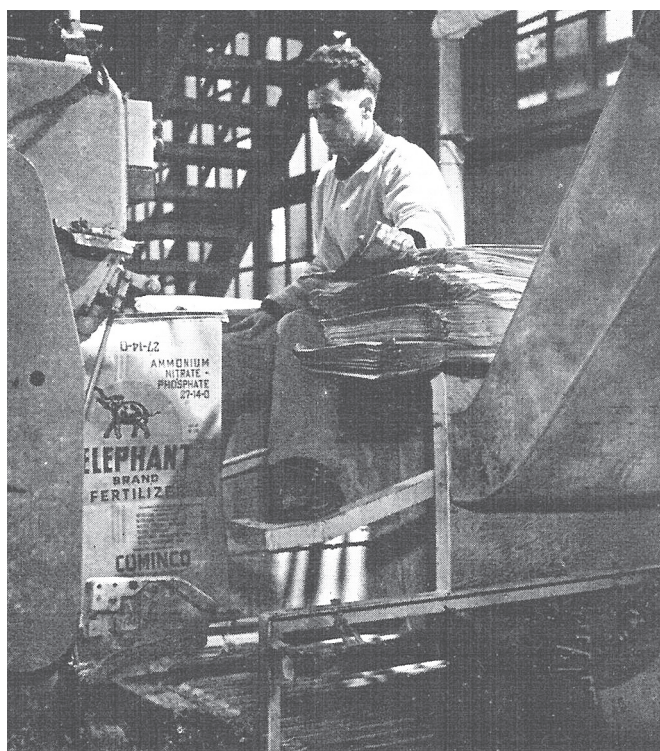
Figure 21: A Cominco worker fills 36-kg (80-lb) bags with ammonium nitrate fertilizer (Cominco 1960, 21)
