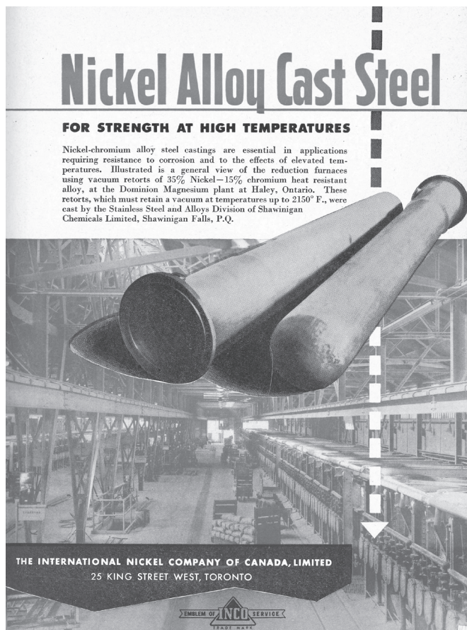
Figure 10: An advertisement for Inco nickel alloy steel. This advertisement shows the vacuum retorts used in the Pidgeon process for producing magnesium (see p. 98). (Inco 1947, 5)
